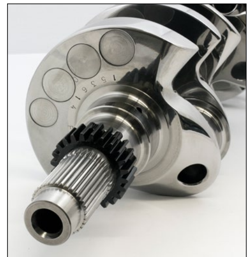
Top Fuel Hemi with Aero-Shed super finish and splined post.
