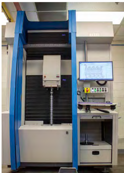
Jenoptik Opticline inspection machine
