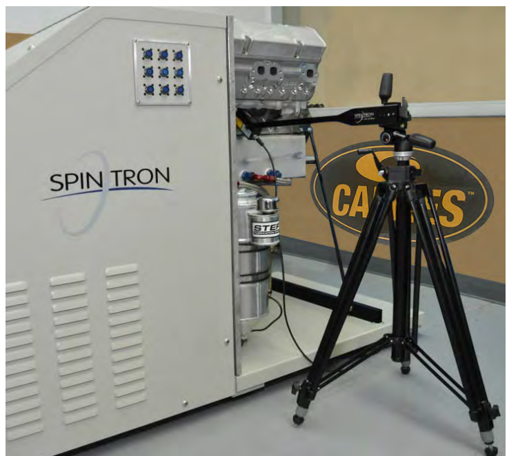
Spintron test rig with laser tracking system
